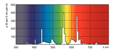
LDPO\_TL5ESS8\_ESS\_840-Spectral power distribution Colour
